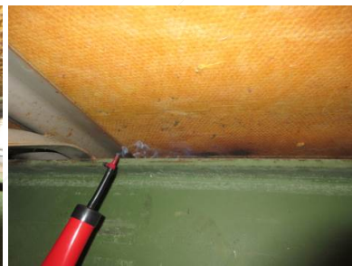
Roof/wall joint leakage diagnosed with Air-Current Tester
